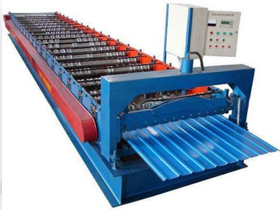
Roof Sheet Rolling
